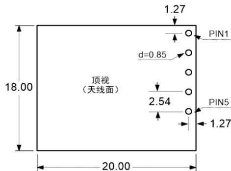
picture4.2 MR5G21Module dimension drawing (unit:mm)
