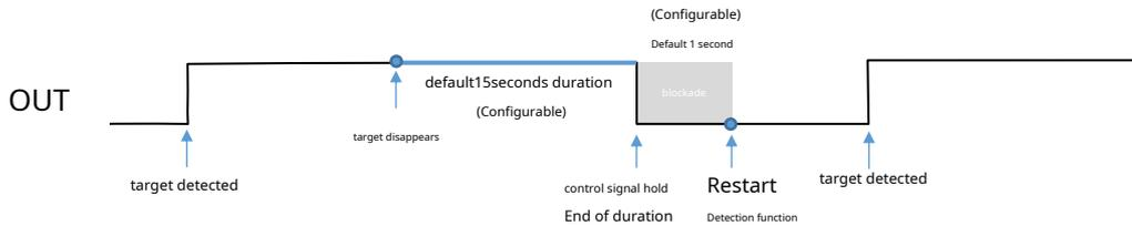
picture5.2 Detection target: OUT Pin Out Signal Timing Diagram
