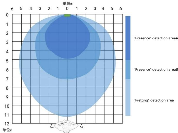
picture3.2 Wall Mount: MR5G21 Schematic diagram of the detection area of the module (the human body faces the module (green rectangle))
