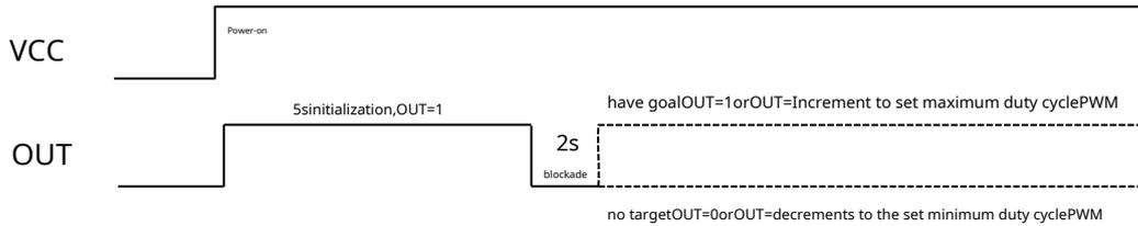
picture5.1 Power-on: OUT Pin Out Signal Timing Diagram
